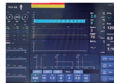
12" TFT LCD screen Displays the Ventilation parameters, Alarm information and Oscillogram.
